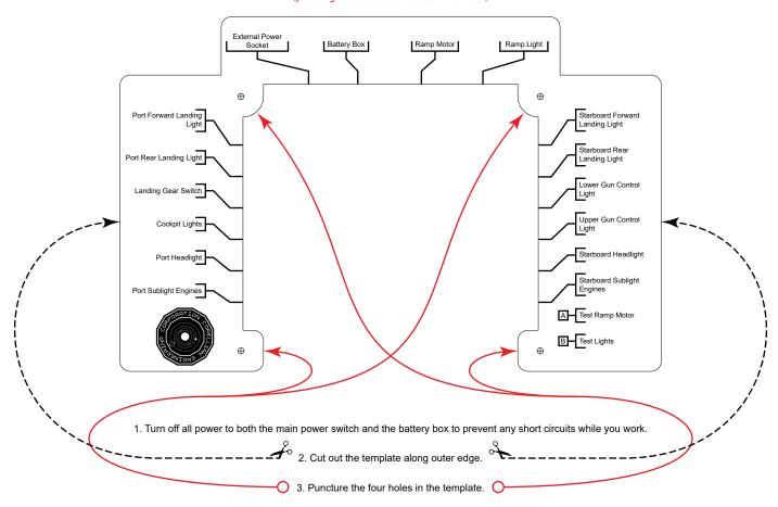
4. If you've already secured the circuit board, carefully remove the screws. Align the template onto the circuit board, and screw it down with the four screws as shown in the diagram.
